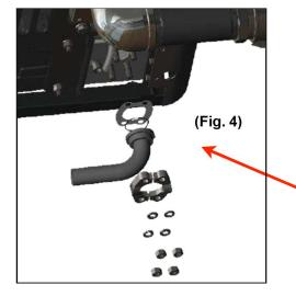
Do Not use power tools to tighten suction fitting.
