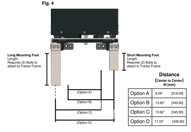
4. Tighten all Mounting Foot bolts at location (c)
