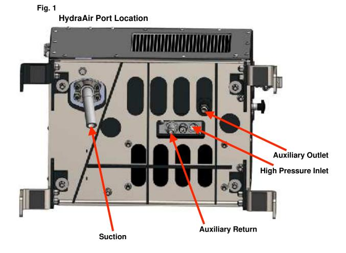
The HydraAIR requires a minimum of 4" clearance from any obstruction or surface.
